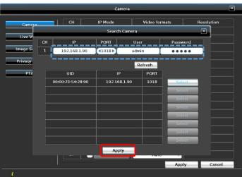
**Step 5.** Go back to the camera page, the selected IP camera applied to the channel already. Click **Apply** and **OK** to save the settings.
