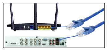
Prepare the DVR, router, and network cable. and connect them as shown in the diagram above.
