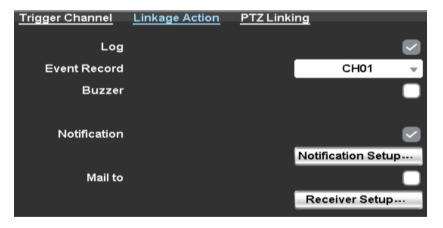
Event Record: Set up the linkage record channel. If motion is detected on channel one, also record on channel three.
