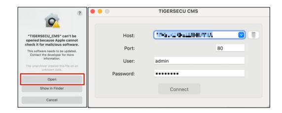
If the CMS shows connection failed, go to the DVR Main Menu, Network Menu, make sure network type shows DHCP and there is a valid IP address. Proceed to the QR Code page to confirm whether the status shows On. If yes, reenter the UID number in the host field and attempt the connection again.
