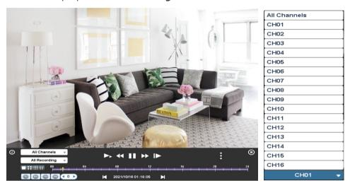
(3) Playback Control Bar. If the playback control bar disappears, move your mouse to the bottom of the window.
