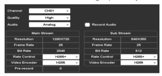
Check **Record Audio** (sound pickup devices need to be purchased separately and connected to the DVR) if you want to record audio for the channel. Switch Audio from **Analog** to **Coax** if the BNC camera has a built-in microphone.
