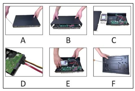
Ensure the DVR is unplugged and removed from main power.
