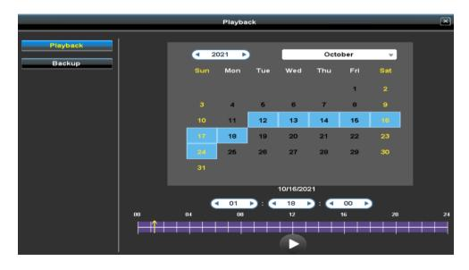
② Here's the **Playback interface**. **All Recording** (Continuous + Event) timeline is marked in purple. **Event Recording** timeline is marked in blue.
