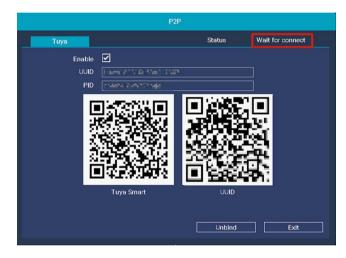
At the P2P screen, enable the **P2P Setting** to allow your NVR's unique QR code to be scanned by your mobile device and permit remote access to your security system.
