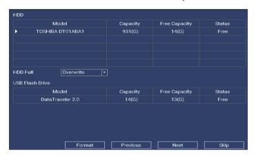
Your recorded video files are stored on your NVR internal hard disk drive (HDD). Formatting the HDD deletes all saved files. It is recommended to format any newly installed HDD before recording.
