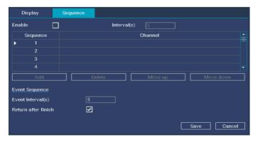
Select **Enable** to activate Sequence Mode. Choose **Add** to add the specific channel(s). Use **Move up/Move down** to adjust the channel sequence. You can also set up Event Tour, which allows the NVR to run auto-sequence if an event occurs.
