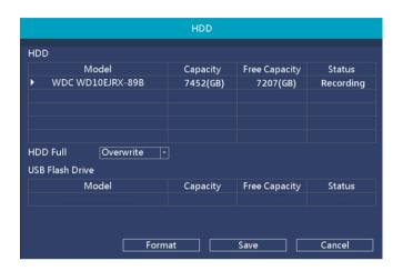
This DVR supports a maximum capacity HDD of 16TB. CAUTION: Formatting the HDD deletes all saved files.
