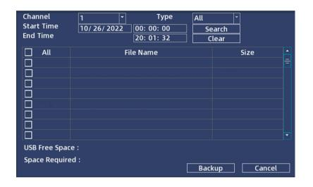
Insert a USB flash drive to the USB slot on the back of the DVR to back up your files.
